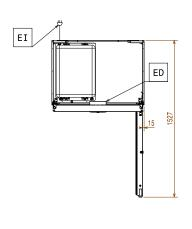
Electric Supply voltage: 220-240 V/1 ph/50 Hz Electrical power, max: 0.45 kW Capacity: Number and type of grids (included): 5 - 530x700 **Key Information:** Net Volume: 510 It Door hinges: External dimensions, Width: 900 mm 700 mm External dimensions, Depth: External dimensions, Depth with 1527 mm
